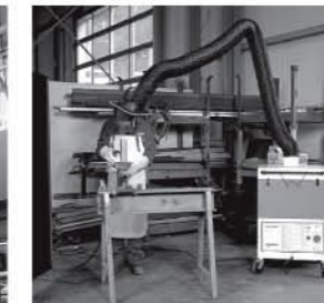
Left: Portable welding fume extraction system
